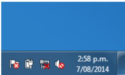
When the icon looks like this, your Ethernet cable going from your computer to your POE injector is either unplugged or the injector is off. Check to be sure that the cable is securely plugged in to the back of the computer and the LAN port on the POE injector. Also check that there is a light on the POE injector and that it is turned on. If the red cross disappears you will have internet connectivity restored.
